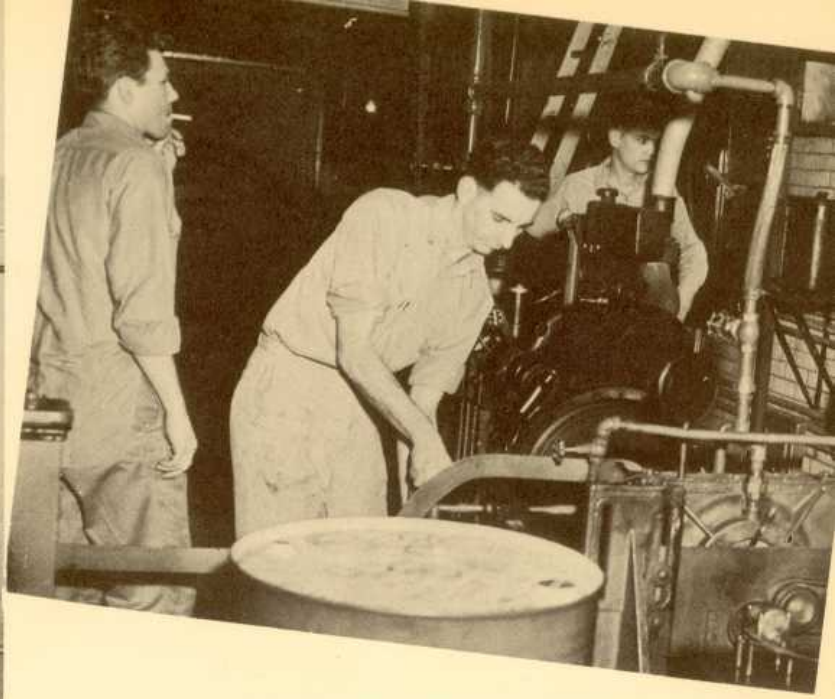
AN ENGINEERING student grabs a quick cigarette as he, with other students, conducts an economy test of the Deisel Engine in the Towne School.
